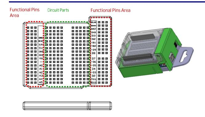
As shown in the figure above is a breadboard, and there are many jacks on the breadboard. Every five jacks in the component plug-in area are connected in a horizontal row.
